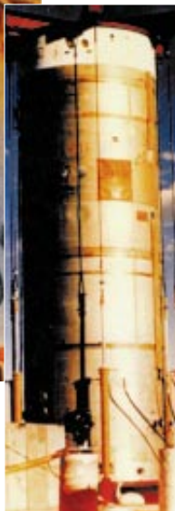
TEST OF THE MIRACL LASER was done on a Titan missile stage, which before exploding dimpled just above the halfway point, where the laser hit (inset).
