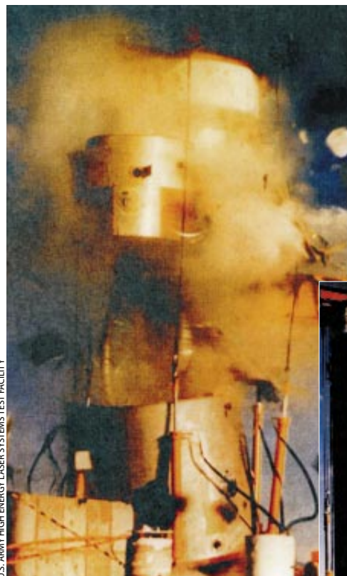
TEST OF THE MIRACL LASER was done on a Titan missile stage, which before exploding dimpled just above the halfway point, where the laser hit (inset).
